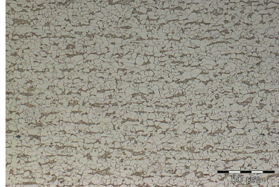
Fig. 1 Microstructure of Dual Phase Steel; white phase : martensite, darker phase : ferrite
