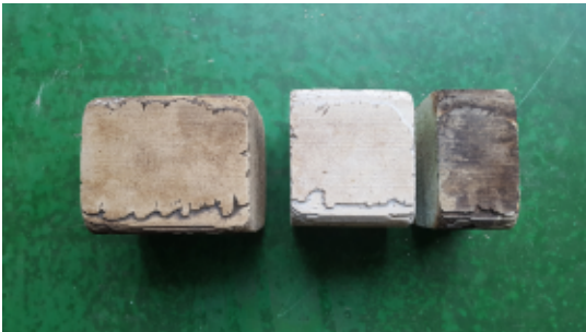
(b) NGOC-LNT-SCR after-treatment catalysts
