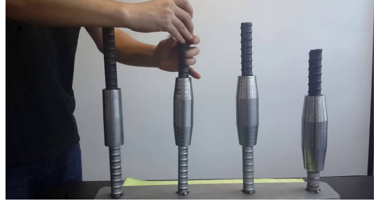
Fig. 3 Rebar's connection of one-touch coupler
