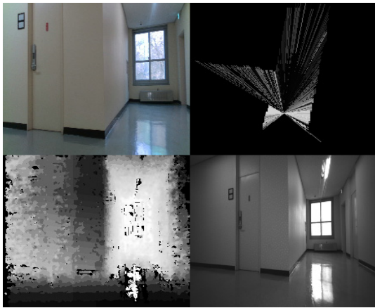
Fig. 2 An image of the training dataset in which pre-processed data are arranged in a grid ((a) top-left: color image, (b) top-right: LiDAR visualization image, (c) bottom-left: depth image, (d) bottom-right: IR image)
