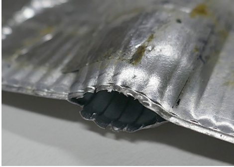
Fig. 3 Ruptured thermosiphon(@90 W)
