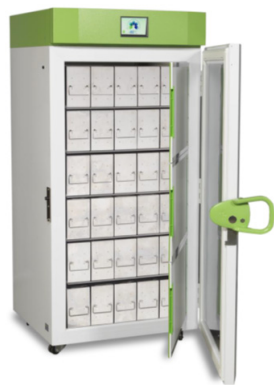
Fig. 1 Ultra-low temperature freezer with Stirling cooler(SU780XLE, Stirling Ultracold)
