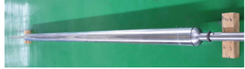
Fig. 5 A mandrel for filament winding
