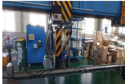
Fig. 12 Filament winding of a composite pipe
