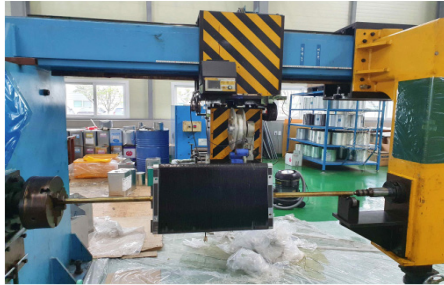
Fig. 8 Winding of a UD composite plate
