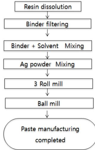
Fig. 2 Preparation process of Ag paste
