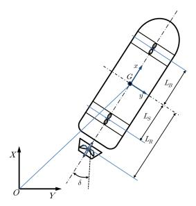
Fig. 3 System description of the controlled ship
