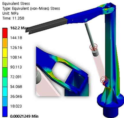
Fig. 8 Equivalent stress contour of small crane at 11.4 sec
