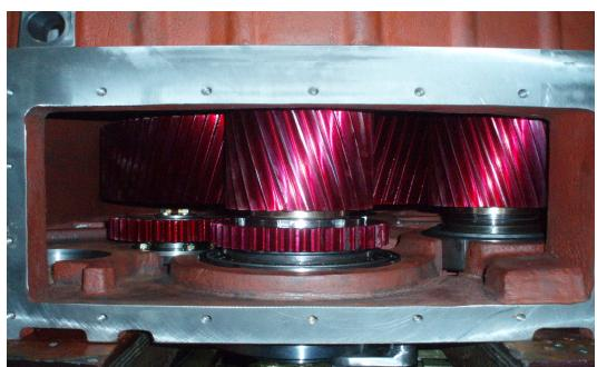
Fig. 7 Photograph of red painted gears for test
