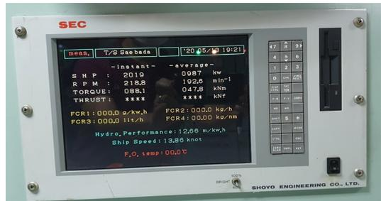
Fig. 3 Ship Performance Monitoring Device
