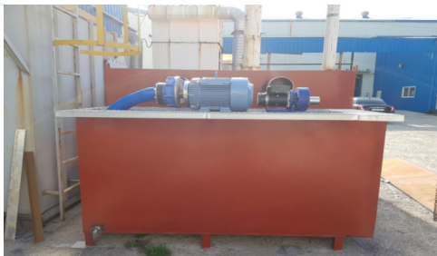
Fig. 6 Thruster pump test bed
