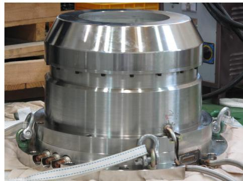
Fig. 8 Oil-cooled stator of the 350 kW motor/generator used in the 35 kWh SFES system
