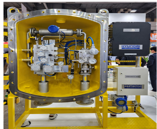
Fig. 1 Designed Gas Valve Unit
