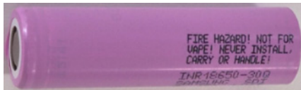
(c) 18650 Lithium-ion battery (Samsung SDI, 3000 mAh)
