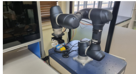
Fig. 7 Oyster transport robot system
