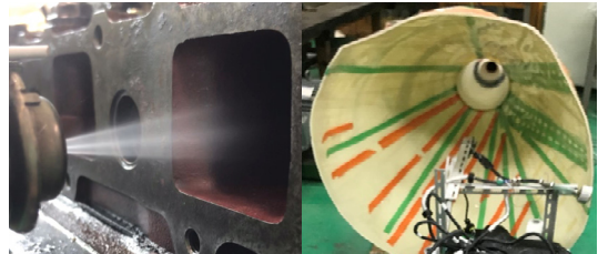
Fig. 7 Pictures of injection test according to position of injector
