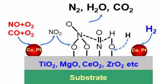
Fig. 6 Mechanism of simultaneous harmful gas reduction of H 2 -SCR
